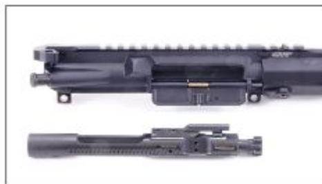
After the breech has been removed, pull the loading lever back to the recess and remove it from the upper housing in the same way as described above.
