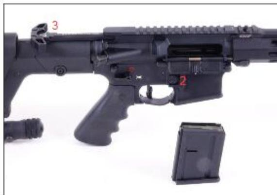
c. Pull the through-loading lever (3) to the rear and look through the right side of the gun through the ejection window and make sure that no cartridge is longer in the chamber. When you pull the bolt catch lever on both sides, the bolt is in the rear position and you can check with your finger whether the chamber is free.
