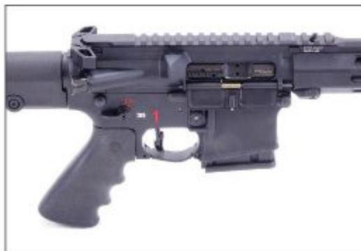
b. Remove the magazine from the weapon, if inserted. Since your weapon is ambidextrous, use the left or right magazine release button (2). Hold the magazine, as it may fall out of the magazine well.
